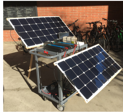
2.5 kW mobile BESS cart with 200 W PV
