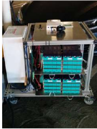
8.7 kW mobile Battery Cart
