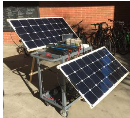
2.5 kW mobile BESS cart with 200 W PV
