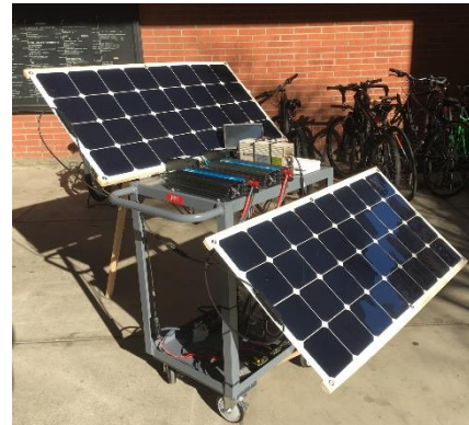
2.5 kW mobile BESS cart with 200 W PV
