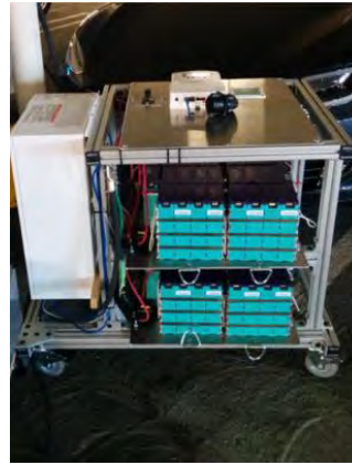
8.7 kW mobile Battery Cart
