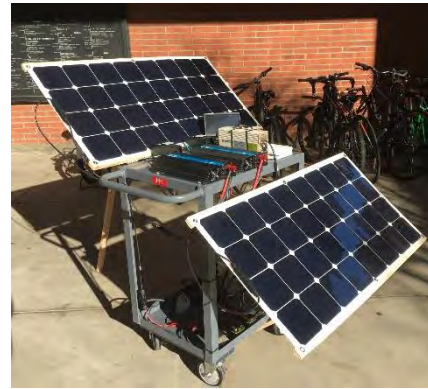
2.5 kW mobile BESS cart with 200 W PV
