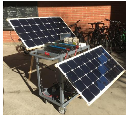
2.5 kW mobile BESS cart with 200 W PV
